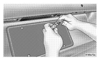
Removing Bulb From Socket **Center High-Mounted Stoplight**
